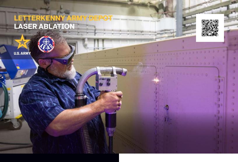
Laser ablation is a subtractive manufacturing technology that utilizes pulsed laser energy to rapidly remove paint and corrosion from solid surfaces by heating and evaporating unwanted materials.
